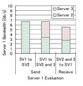
Figure 11. Measured network bandwidth of inter-server communication. SV is server.
