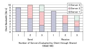
Figure 9. Measured network bandwidth in I/O sharing environment.
