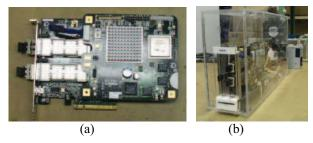
Figure 5. Prototype for I/O device sharing. (a) ExpEther bridge in I/O device side with functions for I/O sharing. (b) I/O box.
