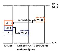
Figure 4. Allocating VF to individual computer by address translation. VF A is allocated to computer A as VF A' and VF B is to computer B as VF B'.
