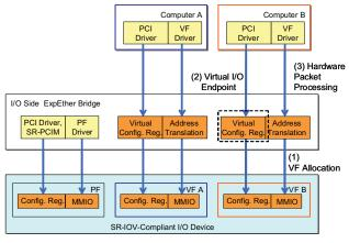
Figure 3. SR-IOV-compliant I/O device shared among multiple computers.
