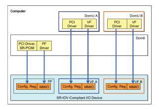
Figure 2. SR-IOV-compliant I/O device used in Xen environment.
