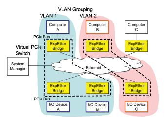
Figure 1. System with ExpEther. Virtual PCIe switch is configured within grouping VLAN. For example, computer A has 1:2 switch and computer B has one of 1:1.
