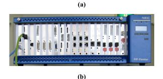
Fig. 4. Developed devices: (a) PEB card, (b) I/O concentrator.
