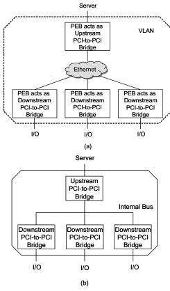
Fig. 3. Block diagram of (a) PCIe switch over Ethernet, (b) conventional PCIe switch.
