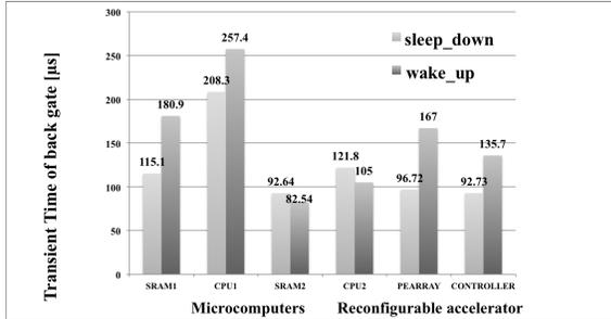
Fig. 1: A transient time of back gate bias from real chip evaluation
