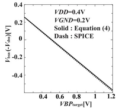
Fig. 6:  $V_{bsn}$  vs  $VBP_{target}$
