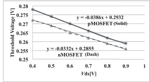
Fig. 4: Threshold voltage vs Drain-Source voltage
