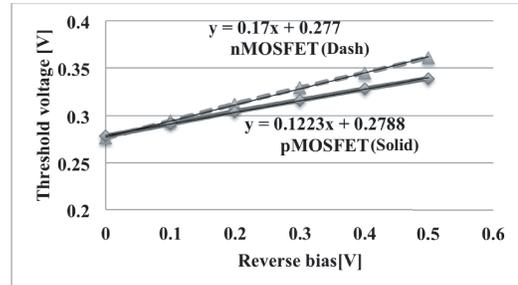
Fig. 5: Threshold voltage vs Reverse bias voltage
