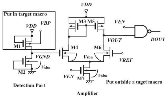
Fig. 2: Structure of a proposed leakage current monitor (this can detect a end of VBP change)
