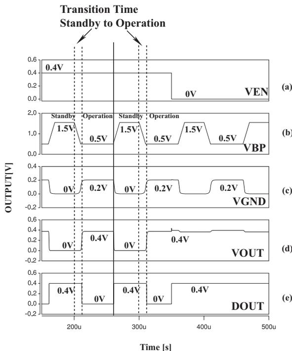
Fig. 3: Waveform of leakage current monitor(VBP detector)
