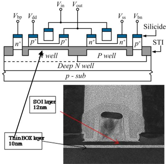
(a) Cross-sectional view of Core and SRAM regions of 65nm SOTB technology
