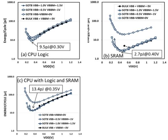
Fig. 6 Measured Energy per cycle values of CPU for Bulk devices and SOTB devices. (a) Energy for CPU logic, (b) Energy for SRAM array for CPU, (c) Total energy for CPU.
