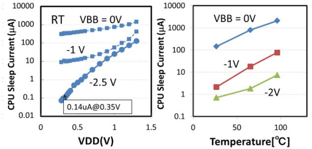
Fig.7 Measured sleep current of CPU on SOTB
