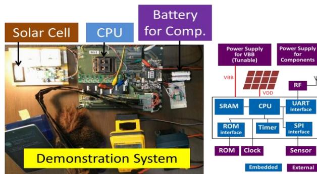
**Fig.10** A picture and block diagram of the demonstration system.
