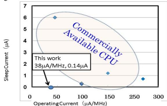
Fig.8 Mapping for sleep current vs operating current
