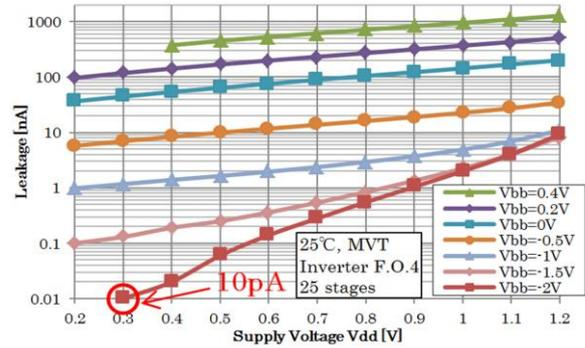
**Fig.2** Measured leakage of a ring oscillator on SOTB devices. The ring oscillator consists of 25-stage FO4 inverters.
