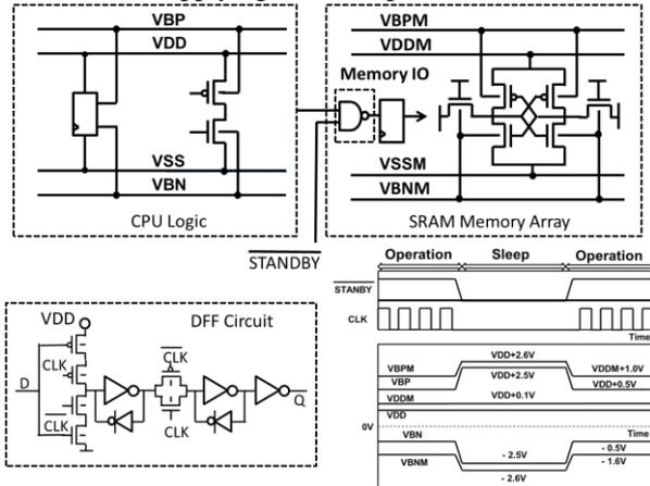
**Fig.3** Structure of power lines of CPU, circuit of DFF, and schematic operating waveforms of CPU.
