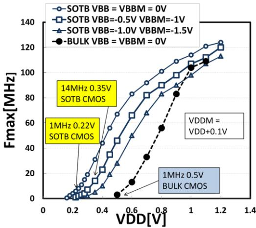
Fig.5 Maximum operating frequency of CPUs by bulk and SOTB, where VBB is parameterized for SOTB.
