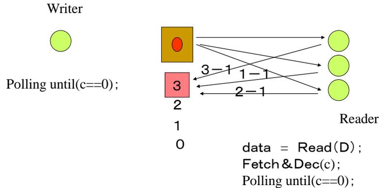
The convenient operation is Fetch&Dec. It reads the data and decrements it indivisibly. The counter can be directly the target of this operation. So, multiple readers problem can be easily solved without using the critical section. The fetch and decrement has two implementations, one is saturated and the other is non-saturated. In the case of saturated, if the reading value is zero, it is not decremented anymore.
