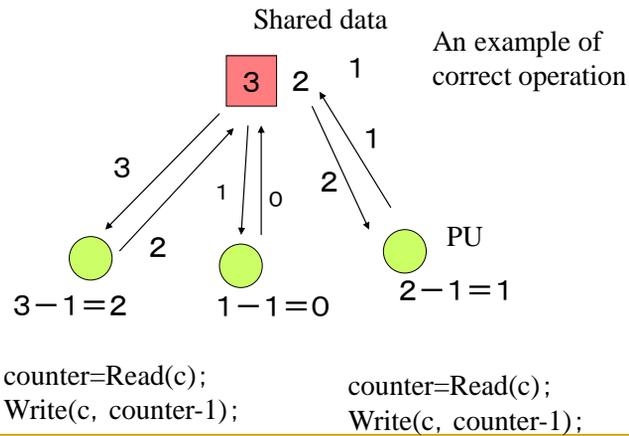
This slide shows the case without any problem. If the Processing Unit accesses the counter in order, it does not cause any problem.
