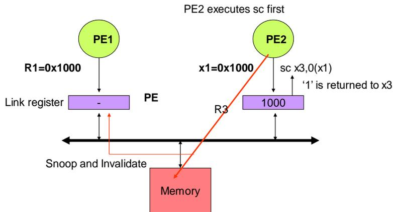
When a PE executes store conditional, the link register is cleared if the address matches. If the link register is alive, it can get 1.
