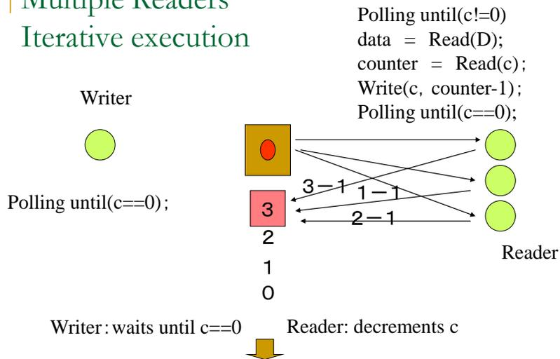
The reader can recognize that the written data are available. So, after reading the data, it decrements the counter. When all readers finish to read, the counter becomes zero. The writer waits for the counter being zero, and then it writes the next data if needed. This operation seems to work well. But, there is a problem, since it introduces the mutual exclusion problem.
