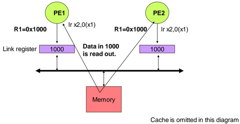
When `lr` is executed, the address is set in the link register attached to each processing element.
