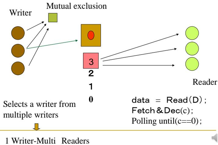
Once the critical section can be used, multi-writers problem can be easily solved. First, a writer is selected with a mutual exclusion operation by using Test and Set for example. Then, the writer executes the single-writer multiple readers problem.
