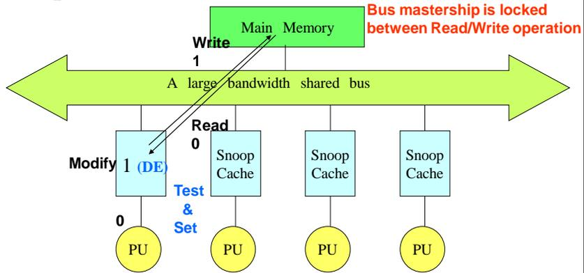
Next, let me explain how the synchronization operations are implemented on the system with private or snoop cache. For example, when Test and Set is implemented on a multi-core system with snoop cache that I explained in the previous class, it will read the main memory and write it locking the bus. Apparently, the value becomes DE since this operation accompanies the write operation.
