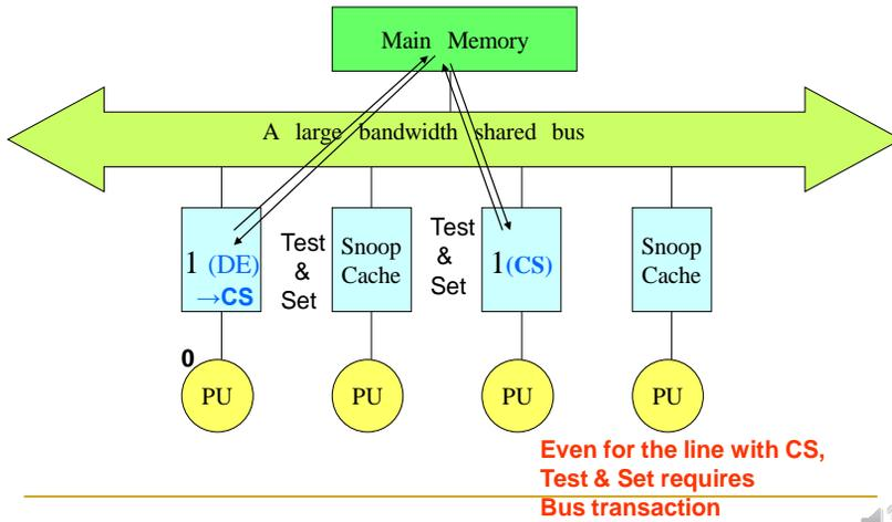
If multiple PUs try busy waiting, bus will be congested because multiple PUs try to access the bus for the Test & Set operations.
