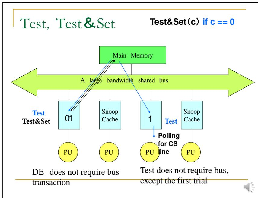
Just by reading the synchronization variable before executing the atomic operation, we can avoid this bus congestion. It is called test test & set. When reading data from the main memory is 1, it is hopeless to try the test and set. In this case, try just reading again.
