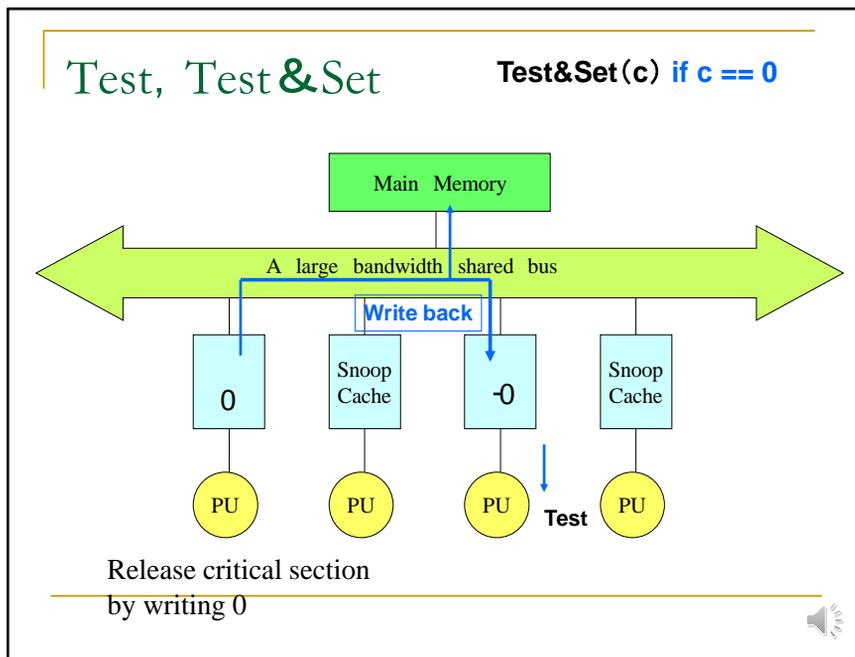
When other PUs reads the synchronization variable. Since it was invalidated, it causes cache-miss, and the value 0 is transferred from the cache which released the critical section. Since the requesting PU gets 0, it executes Test&Set operation. Of course, there may be multiple PUs which get the value 0, but they can be resolved by executing Test&Set.
