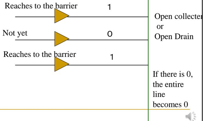
This is an example of the simplest barrier implementation. Only a wire for the open drain output is enough. It is also useful for the debugging.
