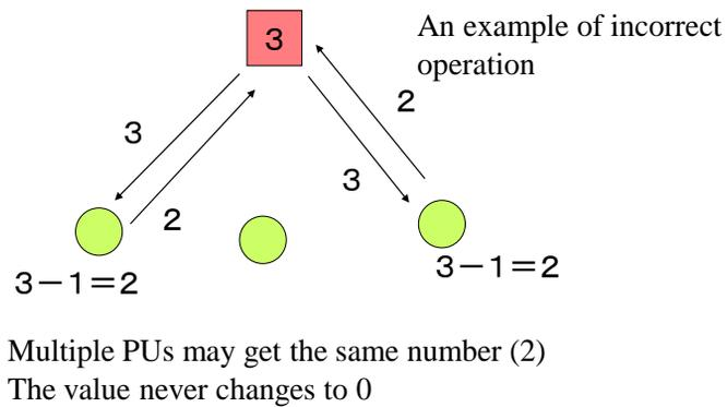
However, what happens when multiple PUs tries to access the counter almost at the same time. When this PU gets three, during it decrements the value, the next PU can read data. It means that two PUs can get the same value 3. In this case, they both write two in the counter, and it never becomes to zero.
