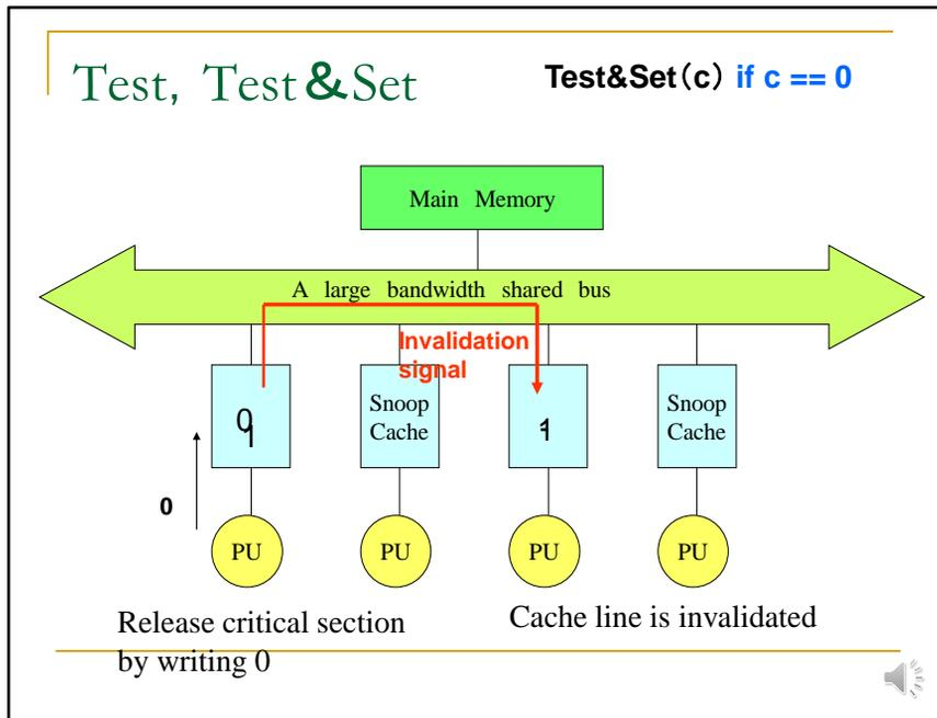
After executing the critical section, a PU writes 0 to release the critical section. At that time, the invalidation signal is transferred on the bus, and other copies are invalidated.
