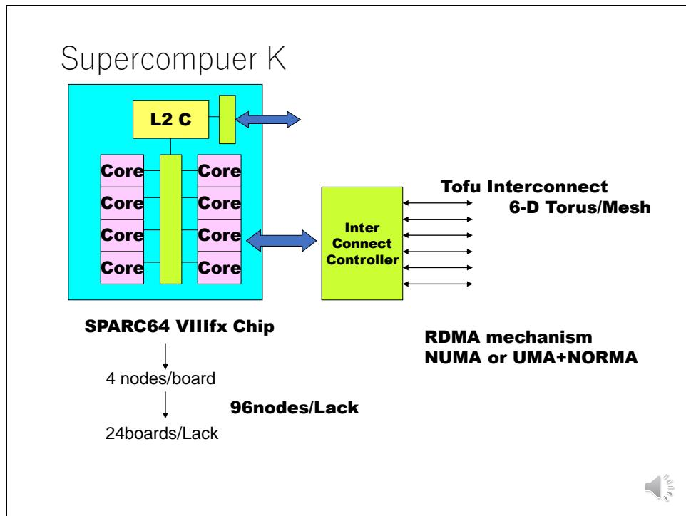
Japanese super computer K uses a simple NUMA structure. It provides Remote DMA mechanism to send the data from other nodes.
