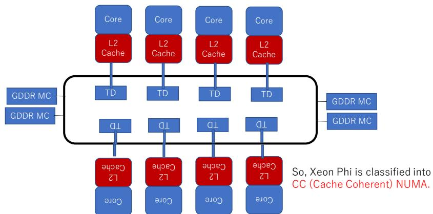
So, Xeon Phi is classified into CC (Cache Coherent) NUMA.
