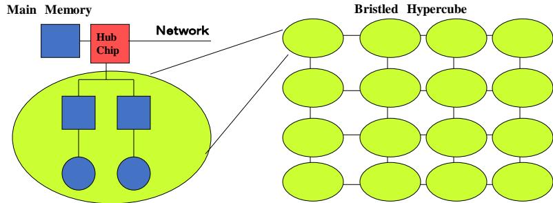
Main Memory is connected with Hub Chip directly.
