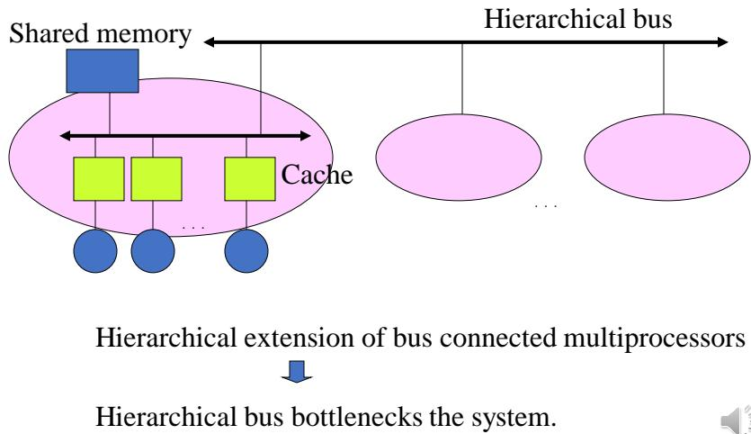
An early CC-NUMA used an extension of the snoop cache by introducing a hierarchical bus. Each cluster was a snoop cache connected multiprocessor, and the accesses for the other cluster uses hierarchical bus. With the similar protocol of the snoop cache also on the hierarchical bus, the cache coherence was kept. Apparently, this approach causes the traffic congestion of the hierarchical bus.
