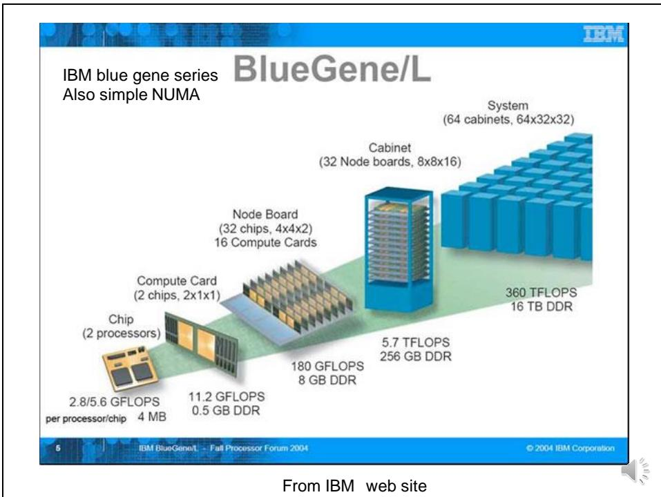
IBM blue gene series BlueGene/L, P and Q also used simple NUMA structure. They are connected with 3-D torus network instead of the crossbar of the earth simulator.
