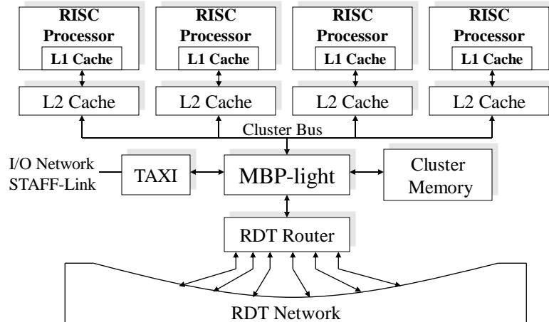
Like a Stanford project, it used a dedicated processor called MBP light for the cache coherent control. 4 SPARC processors are used to develop a cluster, and a special interconnection network called RDT or recursive diagonal torus was used as an interconnection network.
