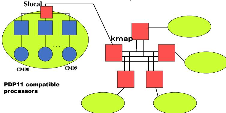
Slocal is an address transform mechanism.
