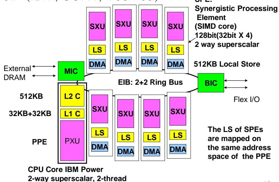
The IBM/SONY/Toshiba developed cell broadband engine for their game machine play station 3. It was also used as several supercomputers. In this architecture, all local memory modules attached to eight SPEs are mapped into the same address space of the host processor address space.
