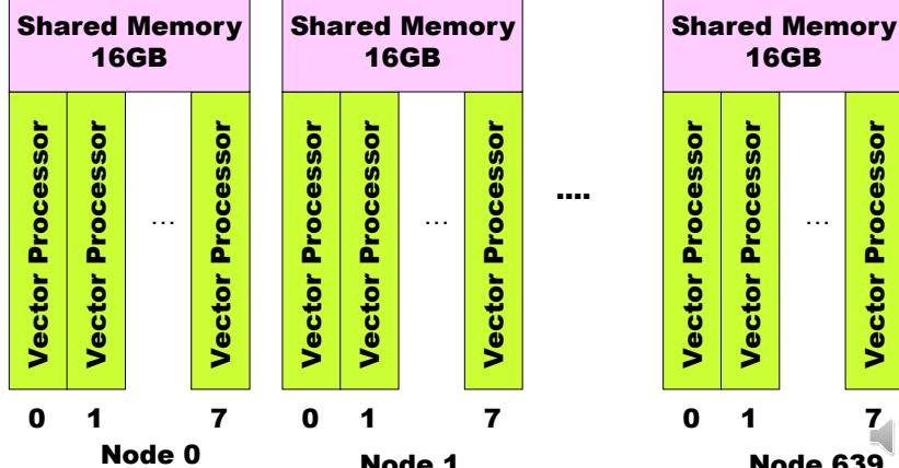
It forms a node with 8 vector processors, and connects 639 nodes with a large crossbar switch. Since the performance of the interconnection network was huge, it achieved an efficient performance close to the peak performance.
