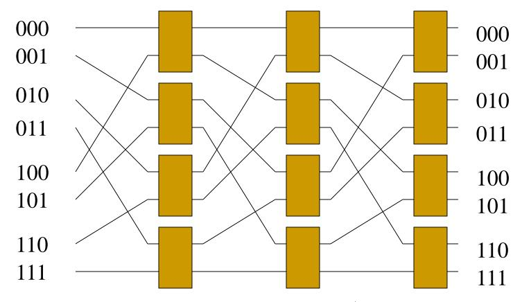
■ The number of switching element (2x2, in this case) is 1/2NxLogN
