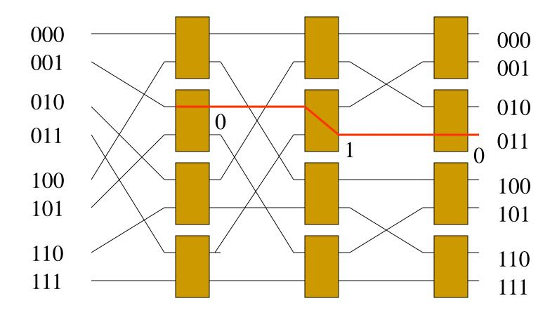
The source label and destination label is compared (Ex-Or): 001→011 Same(0): Straight Different (1): Exchange 010
