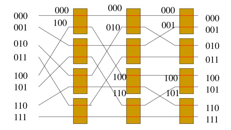
Links labeled with 1bit distance are connected to the same switching element.
