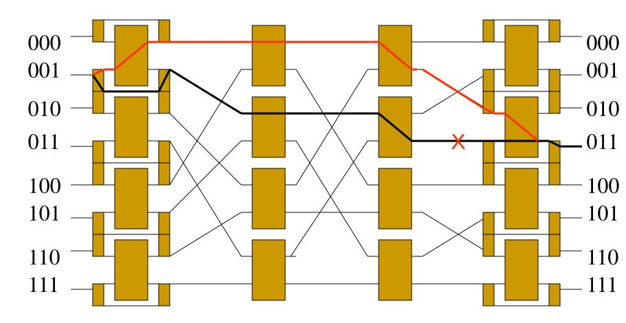
An extra stage + Bypass mechanism
