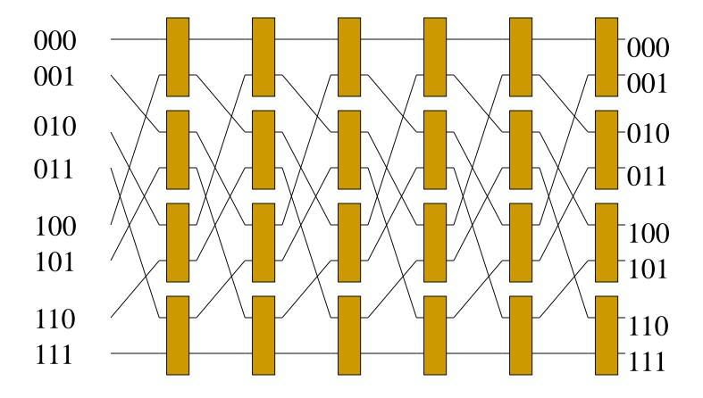
Tandem connection of two Omega networks
