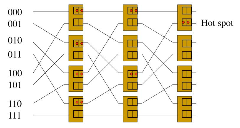
Buffer is saturated in the figure of tree (Tree Saturation)
