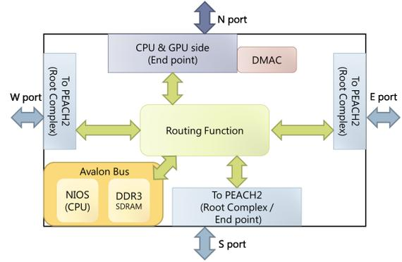
Fig. 2. Block diagram of PEACH2.
