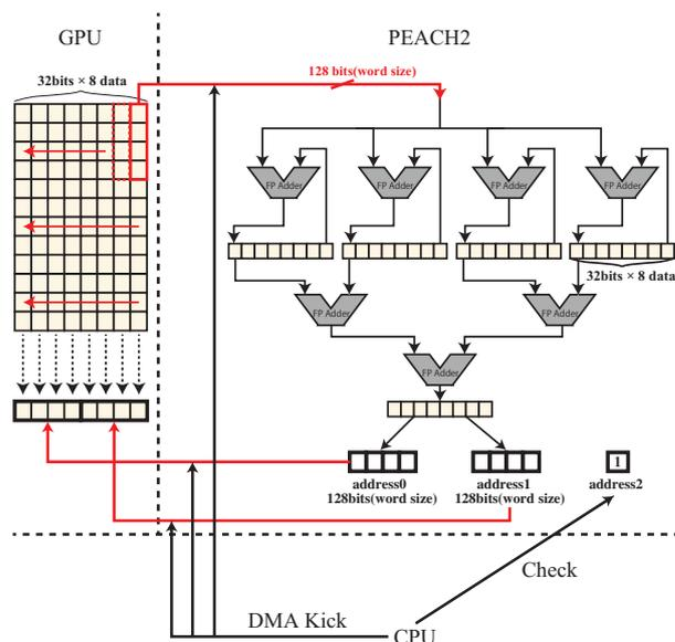
Fig. 5. Block diagram of the reduction calculator
