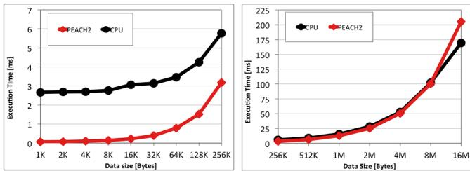
**Fig. 6.** Execution Time vs. Data Size (Left: 1K-256K/Right: 256K-16M)
